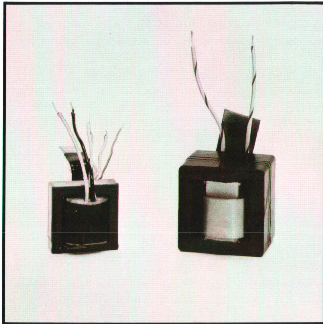
Fig. 7. Efficient cooling also reduced the size of the magnetic components. Main power transformer T1 on the left handles 500 watts with the forced-air cooling. By comparison, the convection-cooled transformer on the right can handle only 200 watts.
